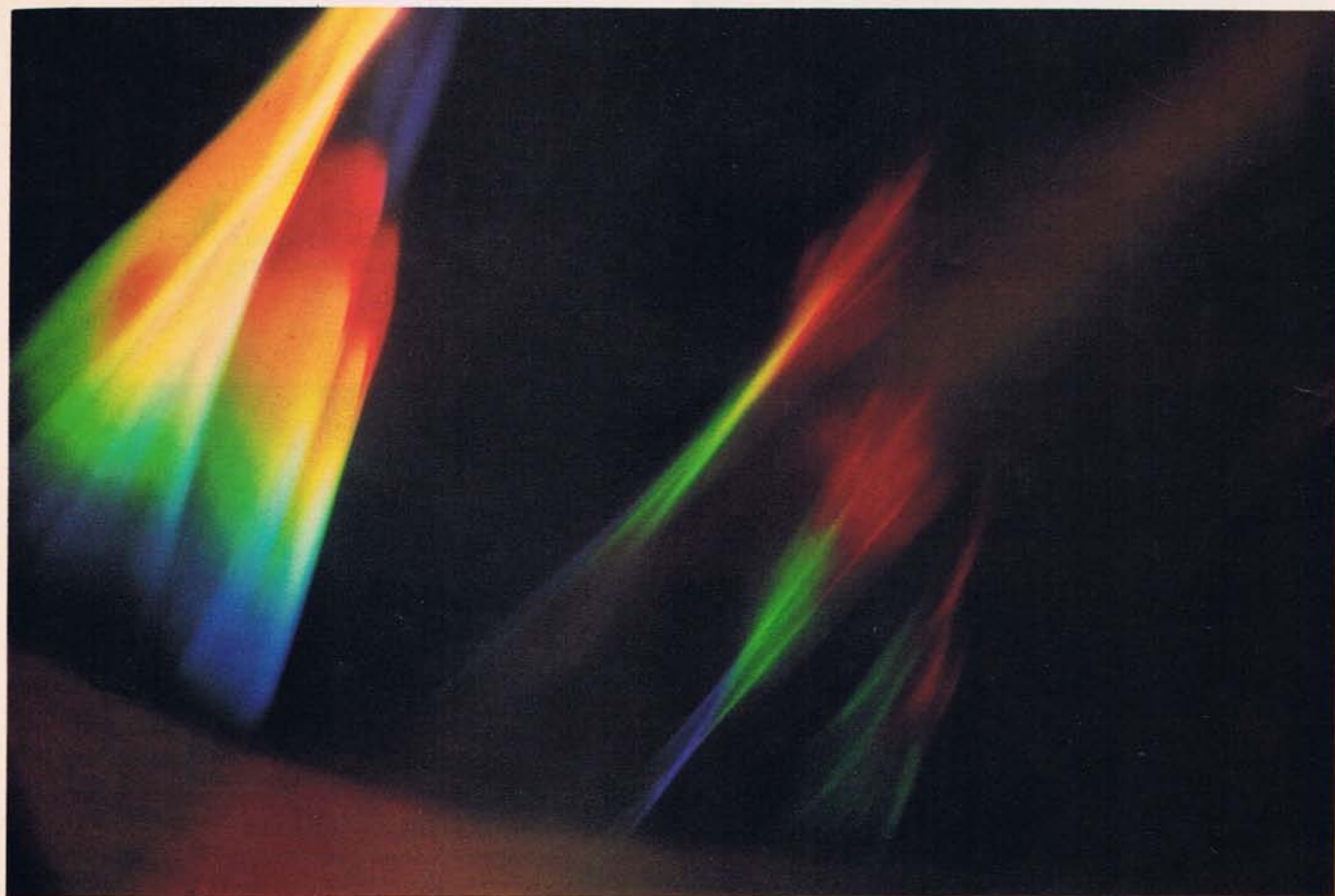
The photograph below is an enlargement of the spectra resulting from directing sunlight on a diffraction grating embossed on Mylar
